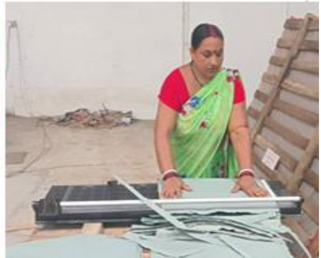
Cluster Artisans processing banana fiber and making 100 GSM and 300 GSM Papers to make varieties of products like BUSINESS CARDS, GREETING CARDS, CERTIFICATE, BROCHURES etc
